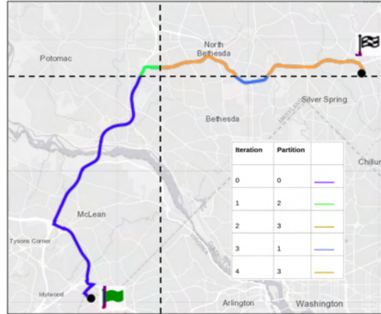
Figure 20: Aggregating the shortest path by back tracking; partition 3 is visited twice from the source located at the lower left partition 0
