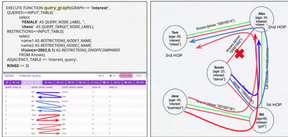
Figure 8: Query-Graph SQL endpoint with OLAP expression support for applying restrictions during many-to-many queries. Column Knows.since that is not captured by the graph unlike columns Knows.name1 , and Knows.name2 , can still be accessed via Kinetica-DB in applying traversal restrictions: Many-to-many query shown in top left finds all the paths from 'Susan' and 'Jane' nodes that are labeled 'FEMALE', to target nodes that are labeled 'chess' within three hops. Restrictions applied on the edges whose 'Person' nodes knows each other since 2002 with the help of 'IF' OLAP function; four paths are found by skipping the restricted edge shown in red cross on right, two from 'Susan' and two from 'Jane' shown in the table interest_query in blue and orange paths, respectively (bottom left).
